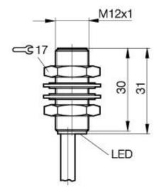
Inductive Sensors BES 516-370-G-E4-Y-03 M12x1 x 31 normally-closed Sn=4mm shielded
